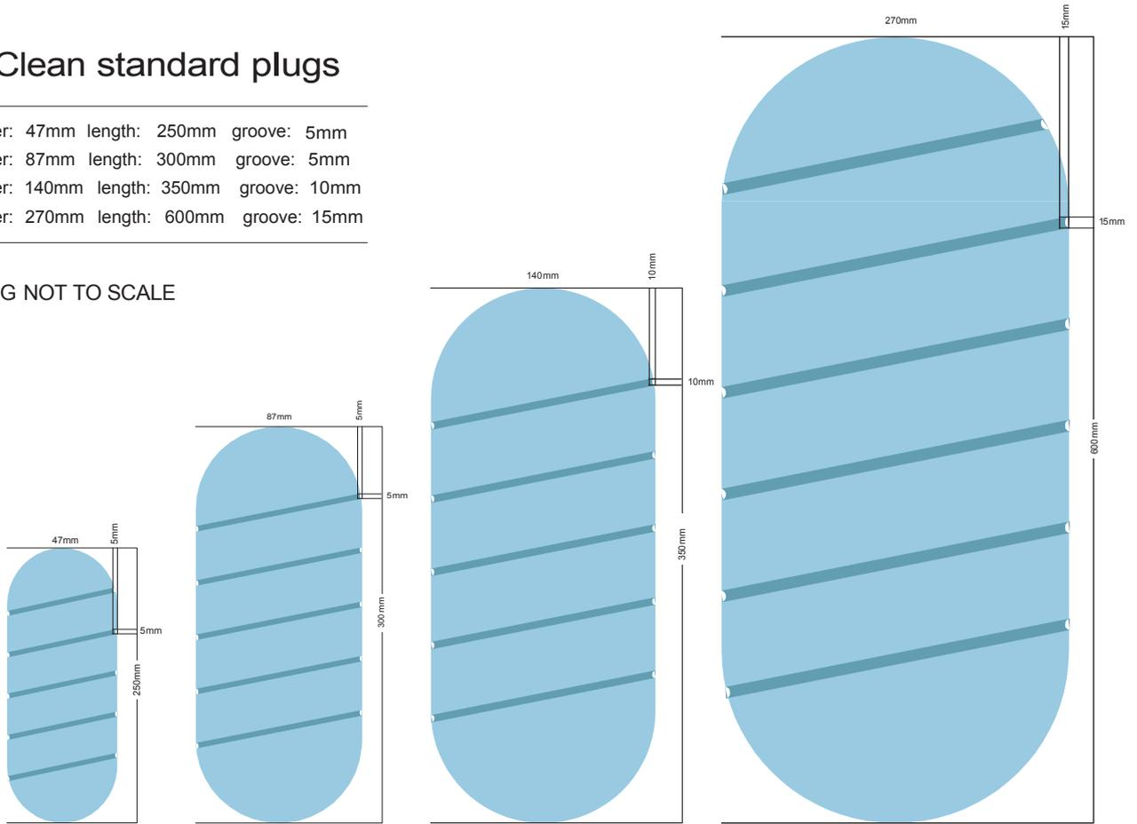
ABOVE: These are the standard existing plug sizes. The foam material they consist of is flexible enough to provide great adaptability between standard sizes. Production runs of other sizes can be custom made to order if needed.
